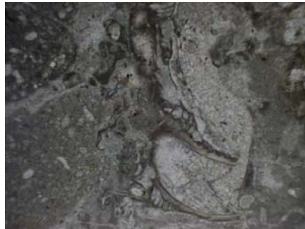
This is the marble at 10x magnification Same image with crossed polars.
